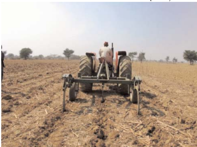
Basic mechanised minimum-till. Cost to client about $50/ha. Time taken one hour per hectare
