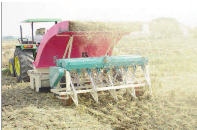
Fig.1 Happy seeder with no-till drill with inverted T type furrow openers
