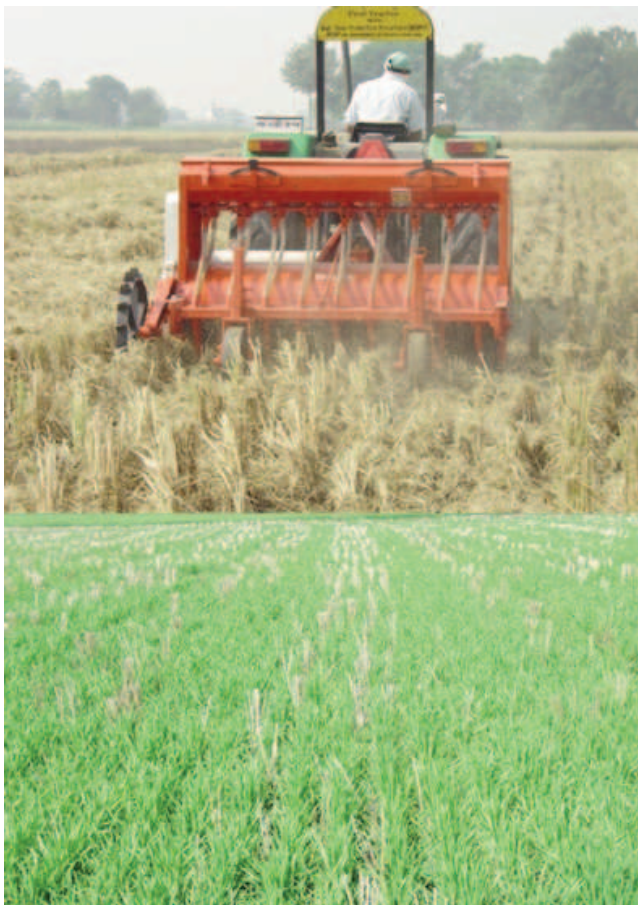
Fig. 3 Turbo HS sowing wheat in rice residue and wheat crop stand in rice residue
